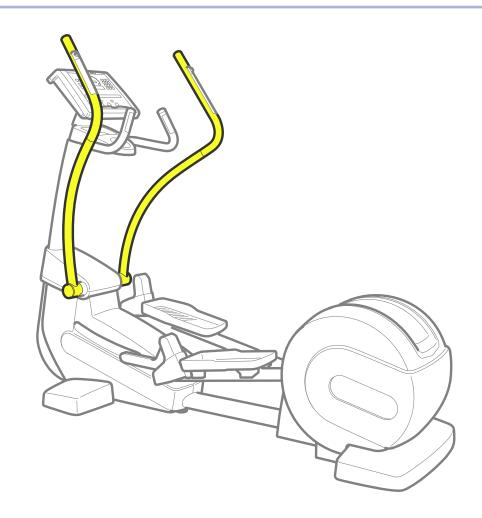
Levers: these can be grasped by the user to perform the exercise with arm movements. The 700 and 700 SP versions have sensors for monitoring the heart rate (hand sensor) and the Fast Track Control to change the effort level.
