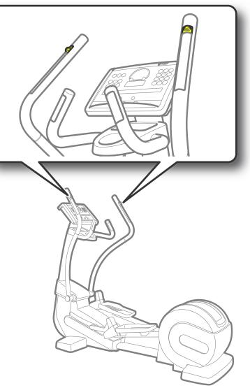
**Levers**: these can be grasped by the user to perform the exercise with arm movements. The 700 and 700 SP versions have **sensors** for monitoring the heat rate (hand sensor) and the **Fast Track Control** to change the effort level.
