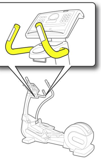
**Fixed handles**: these can be grasped by the user during the workout. The 700 and 700 SP versions have **sensors** for monitoring the heart rate (hand sensor).
